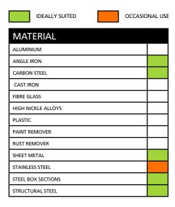
**DESCRIPTION:** Premium flat metal cutting discs that provide an excellent cost / performance ratio across a broad range of ferrous steel applications.
