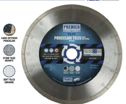
**DESCRIPTION:** The P5-PT is a continuous rim blade which offers fast and efficient cutting through porcelain and other hard interior tiles. Sizes 180mm and above are for fixed tile saws and perform better when used wet
