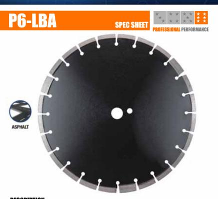
DESCRIPTION: The P6-LBA looping blade is available in **PRODUCT DETAILS**: 350mm diameter with either 8 or 10mm wide segments. They are used on floor saw machines for cutting wide channels in the surface when preparing for the installation of traffic detector loop management systems; this is a sub-surface method of identifying the presence of a vehicle at traffic lights and security barriers.
