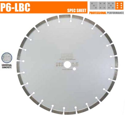
**DESCRIPTION:** PDP's Looping diamond blades are available in 350mm diameter with either 8mm or 10mm wide segments. They are primarily used on floor saw machines for cutting wide channels in concrete or asphalt when preparing for the installation of traffic detector loop management systems. This is a sub-surface method of identifying the presence and speed of a vehicle at traffic lights and security barriers
