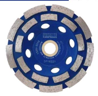
**DESCRIPTION:** Premium double row dimond cup grinder designed to grind away uneven concrete and stone surfaces. Also suitable for preparing a surface prior to polishing or a coating application. The double row of segments provides fast stock removal and good life. The 110mm diameter is for use on the Makita PC1100 concrete planer or 115mm angle grinders.
