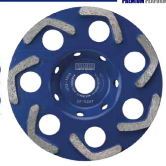
**DESCRIPTION:** The P5-HCG 150mm (6") cup grinder has a 19mm bore to specifically fit the Hilti DG150 diamond grinding machine. The high quality diamond segments have been designed to work at optimum speeds between 4700rpm and 6600rpm, whilst the plate holes provide an ample outlet for dust extraction.
