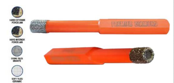
**DESCRIPTION:** Our range of auto-cool diamond tile drills are filled with a lubricating wax. During the drilling process the leading edge of the wax melts and autocools the diamonds, meaning there is no need to apply a secondary coolant, such as water. With hexagonal fitting for use in cordless and corded drills.
