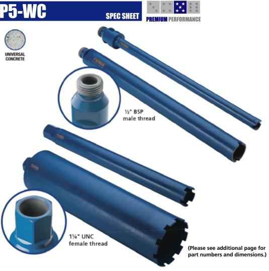
**DESCRIPTION:** The P5-WC wet diamond cores are designed for drilling into concrete and reinforced concrete by using suitable diamond drill motors that run at appropriate speeds. The machine speed is mainly dependent on the core size and strength of the concrete. Ideally a drilling rig stand is recommended as this can be fixed down to ensure there is no movement in the set-up, however for smaller diameters it is possible to use some diamond motors hand held
