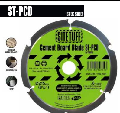
**DESCRIPTION:** ST-PCD is a saw blade with solid Polycrystalline Diamond (PCD) teeth that cut effortlessly through cement fibre boards and many other difficult to cut composite panels. They are designed to be used on wood working machines, such as cordless trim saws, corded circular saws, mitre saws and table saws.
