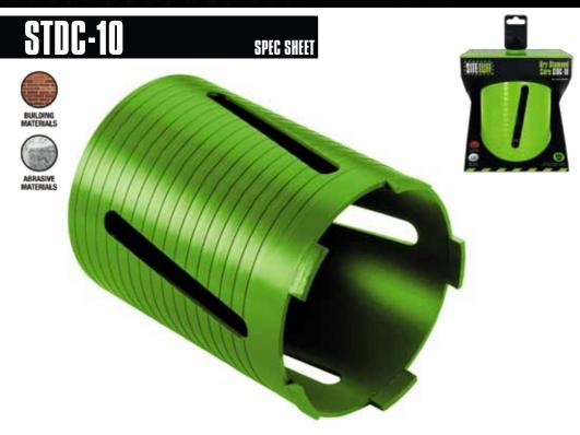
**DESCRIPTION:** The SiteTuff range of dry core drills are designed for use on the most common UK construction materials, including facing bricks and concrete blocks. The counter clockwise spiral on the core body is designed to assist in the dispersal of debris whilst drilling, helping to reduce the risk of the core jamming in the hole
